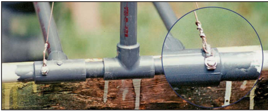
Figure 5 —The crossover feed wires are attached to the element ends with large solder lugs and stainless sheet metal screws. Weatherproof the connection with a blob of silicone sealant.
